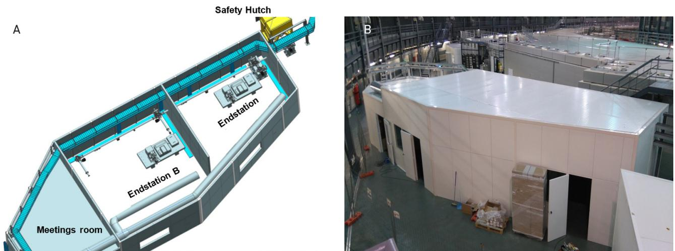
**Figure 14:** 3D drawings of the experimental hutch. There are two endstations hosting the three branches. Two of these branches will be coupled to a FTIR systems as indicated in the figure, the third branch will be a free station, where the users can bring their own instrument and connect it to this branch.
