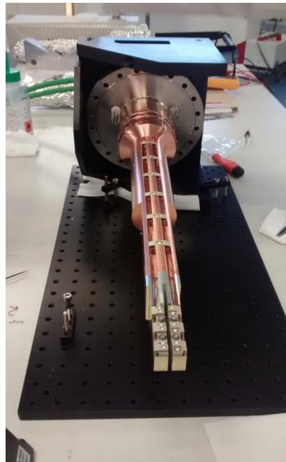
**Figure 16:** Extraction mirror M1 pre-installation. Installation of thermocouples.
